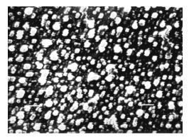
**Figure 1** SEM photomicrograph (×5000) of etched fractured surface for SBS extrudate from the capillary rheometer at 200°C.
