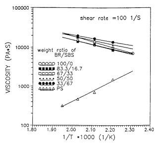
**Figure 6** Temperature dependence of viscosity of the BR-SBS blends and PS at shear rate of 100 S<sup>-1</sup>.
