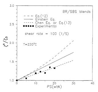
**Figure 12** The relative viscosity predicted by eqs. (1), (8), (12), and (13) and experimental values measured at  $220^{\circ}$ C at shear rate of  $100 \text{ S}^{-1}$ .
