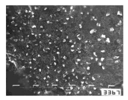
**Figure 2** SEM photomicrograph ( $\times 5000$ ) of etched fractured surface for the BR-SBS extrudate from the capillary rheometer with a weight ratio of BR-SBS = 50/50 (or ST/BD = 15/85) at 200°C.
