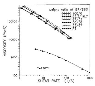
**Figure 5** Viscosity versus shear rate for the BR–SBS blends and PS at 220°C.
