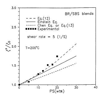
**Figure 7** The relative viscosity predicted by eqs. (1), (8), (12), and (13) and experimental values measured at  $200^{\circ}$ C at shear rate of 5 S<sup>-1</sup>.
