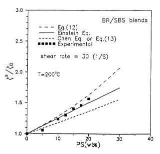
**Figure 8** The relative viscosity predicted by eqs. (1), (8), (12), and (13) and experimental values measured at  $200^{\circ}$ C at shear rate of  $30 \text{ S}^{-1}$ .
