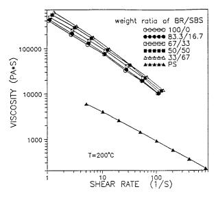
**Figure 4** Viscosity versus shear rate for the BR–SBS blends and PS at 200°C.
