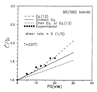
**Figure 10** The relative viscosity predicted by eqs. (1), (8), (12), and (13) and experimental values measured at  $220^{\circ}$ C at shear rate of 5 S<sup>-1</sup>.
