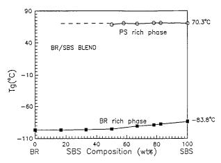
Figure 3  $T_g$  (BR) and  $T_g$  (PS) for BR–SBS blends.
