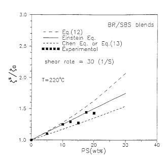
**Figure 11** The relative viscosity predicted by eqs. (1), (8), (12), and (13) and experimental values measured at  $220^{\circ}$ C at shear rate of  $30 \text{ S}^{-1}$ .
