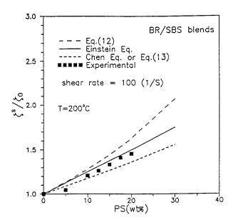
**Figure 9** The relative viscosity predicted by eqs. (1), (8), (12), and (13) and experimental values measured at  $200^{\circ}$ C at shear rate of  $100 \text{ S}^{-1}$ .
